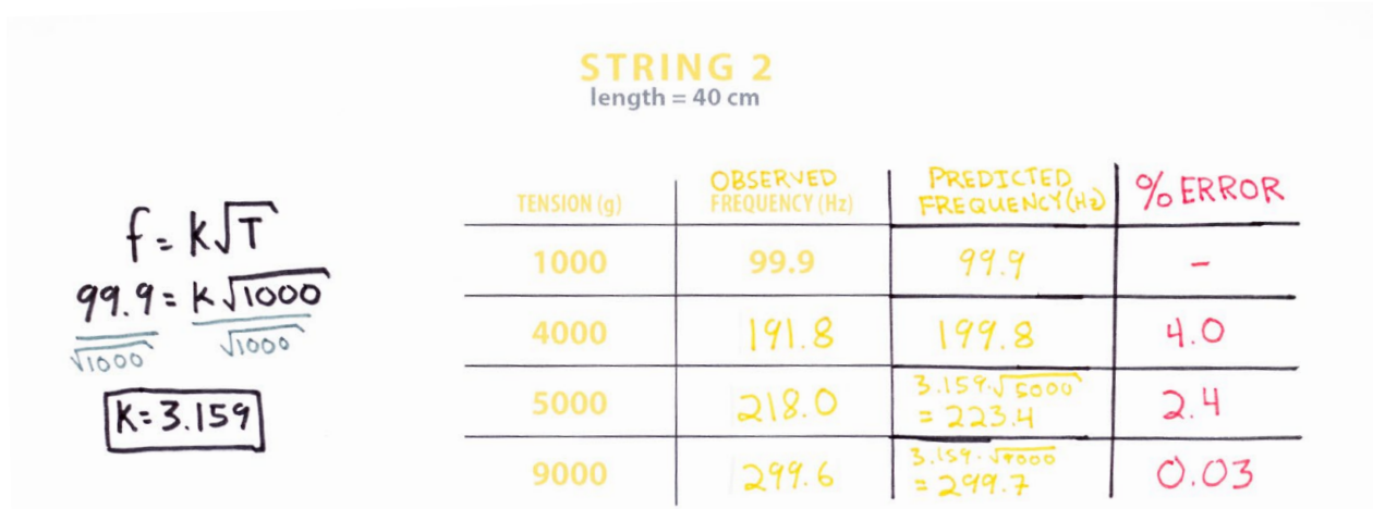
Figure 22 | Our Equation Works! After computing our constant of proportionality k using our single observation at this length and tension - we've made predictions for all string lengths. And when we compare to experiment using our high speed camera - our predictions are quite close to our observations! Booya!
